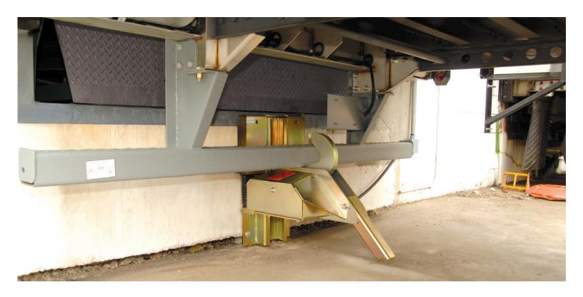
Vehicle restraints were developed specifically to reduce the occurrence of accidents at the dock. The DE2000 rotating hook restraint — our superior, impact-style trailer restraint — combines an advanced communication system with a low-profile carriage. It also has an impact extension bar that accommodates a wide range of lower rear impact guards.
