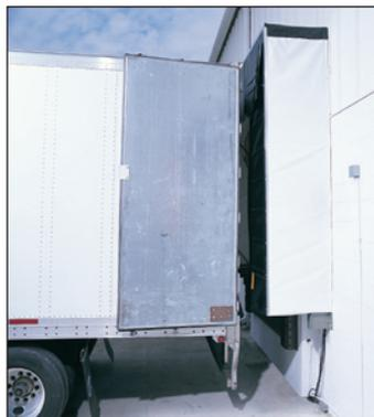
◀ If off-center trailer contact occurs, the S-3200 moves upward and back, preventing costly damage to the wall and shelter. After the truck leaves, a gravity-biased design returns the frame to its original position.
