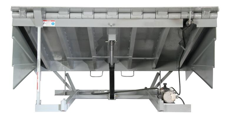
The ASSA ABLOY model DE-H hydraulic dock leveler is pit-mounted and activated by a hydraulic cylinder to raise the leveler and a cylinder that powers out the lip, allowing the unit to then gently descend into position via gravity. The DE-H series dock leveler is designed to provide years of durability and dependability in a variety of loading dock applications where productivity is vital.
